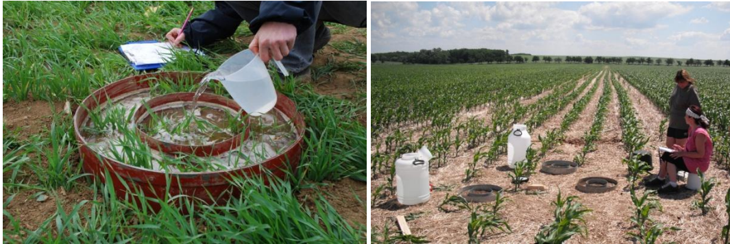
Fig. 1 Photo of the double ring infiltrometers and view at the site with three replications (sets of infiltrometers)
